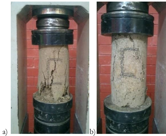
Figure 3. Poured earth cylinders model white or witness, with low failures to Simple compression tests.
