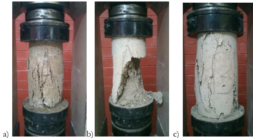
Figure 4. Pilted earth cylinders dosed with lime, with low flaws to Simple compression tests.
