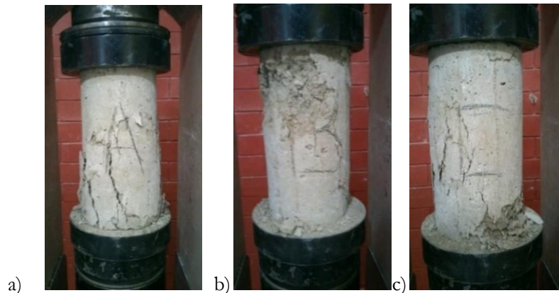
Figure 5: Poured earth cylinders dosed with Portland cement, with low failures to Simple compression tests.
