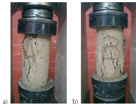
Figure 6: Poured earth cylinders with xanthan gum, with low failures to Simple compression tests.
