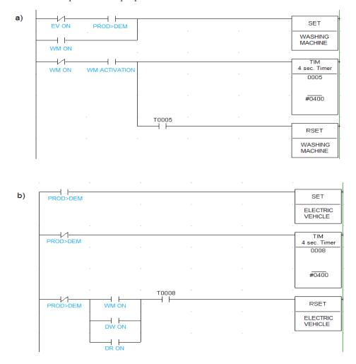
Figure 6.Relay Diagram implemented with CX-Programmer to activate programmable loads (6a for the Washing Machine and 6b for the Electric Vehicle) inside PV Window. 'EV ON' is the contact for the EV (I0.0) to indicate that the vehicle is being charged, to avoid the simultaneous activation of both loads. 'PROD>DEM'
