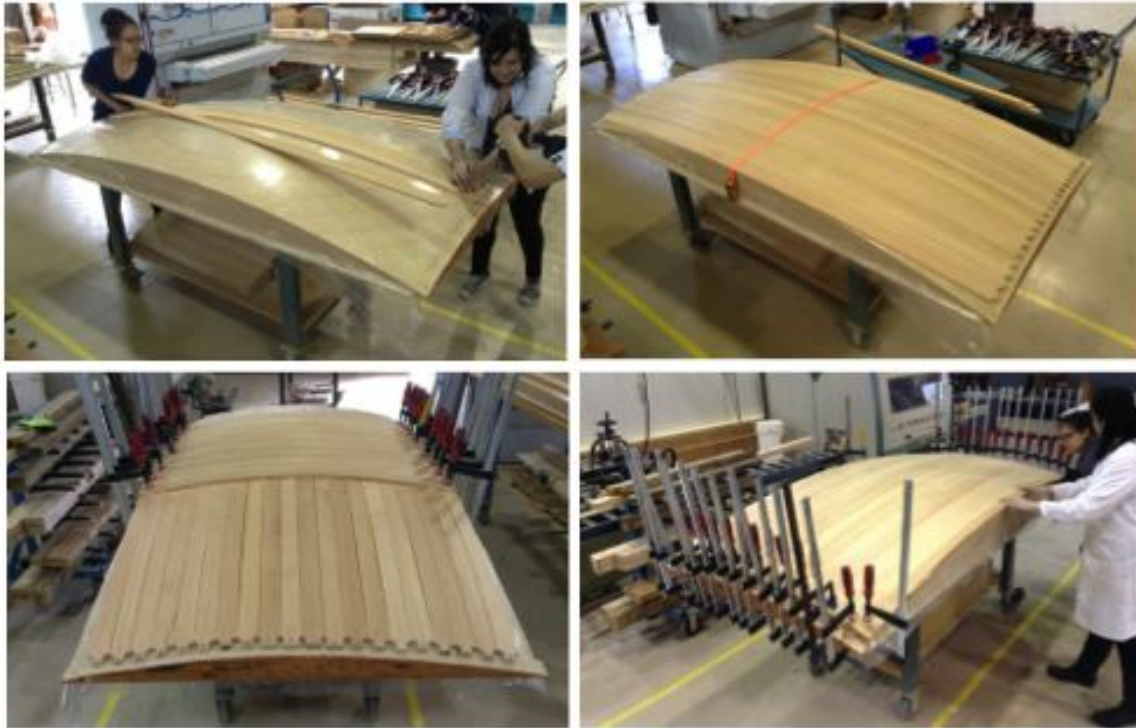
Figure 6: Fabrication of torus shaped element
