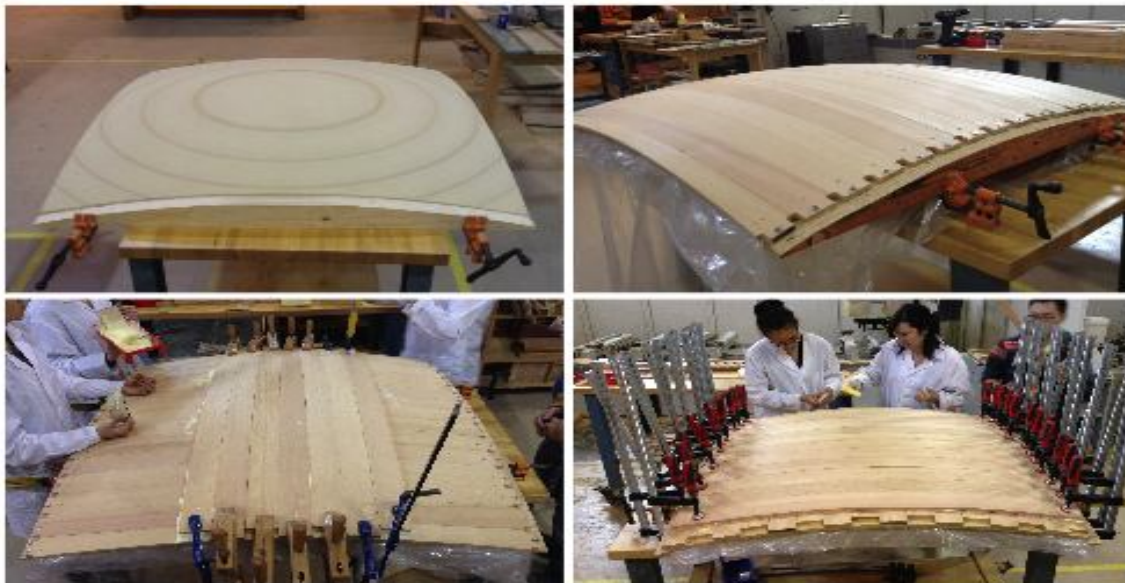
Figure 5: Fabrication of glued prototype with same curvature in two directions
