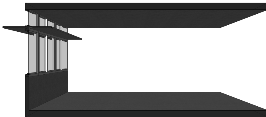
Figure 1: Section drawing of a light shelf system.
