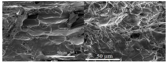
Figure 5. a) Brittle Cleavage (Saffron"),b)Mixed Brittle and Ductile Fracture (11375) at -20 °C
