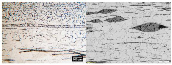
Figure 1: a - Irregular Row Ferritic - Pearlitic Structure, b - Details of Inclusions
