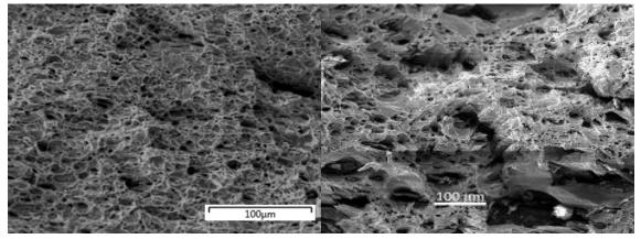
Figure 4: Transcrystalline Ductile Fracture Morphology – a) 11375, b) Saffron
