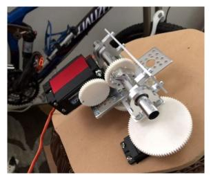
Figure 5: Neck Mechanism
