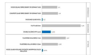
Figure 2: Materials Thermal Transmittance Values (kW/m<sup>2</sup>K)
