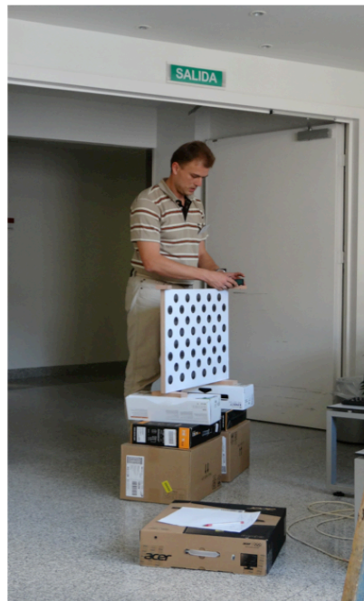
Fig. 16: Calibration Process for Depth Image-based Sensors
