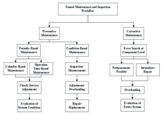
Figure 2. PIARC Comprehensive Tunnel Maintenance and Inspection Workflow
