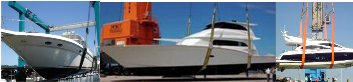
Fig. 1 – Marine slings lifting large boats.
