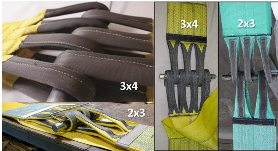
Fig. 2 – Examples of 2x3 and 2x4 disconnect features on web slings.
