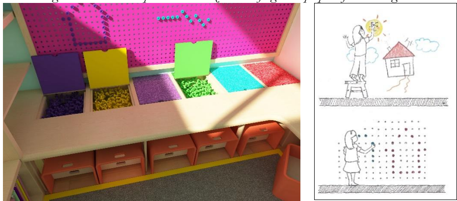
<Figure 27 > Punched metal wall covering to create a tactile experience of painting on the wall
